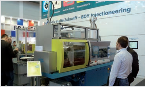
Production cell with CE-compliant safety housing
