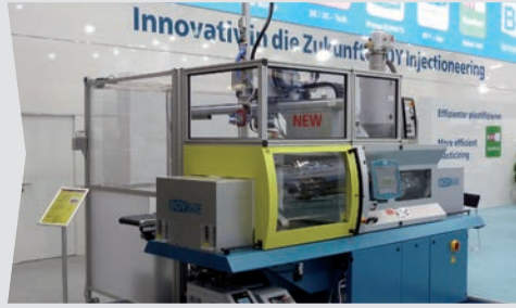
Production cell with CE-compliant safety housing
