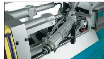
The swivel-out injection unit simplifies the retrofit procedure and maintenance.
