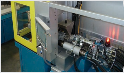
Injection unit for 2C injection moulding tightly mounted on the machine table
