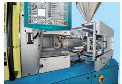
The swivel-out injection unit facilitates alterations and maintenance
