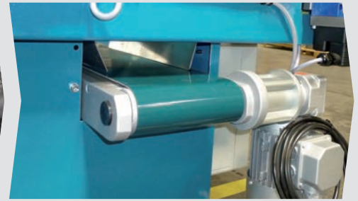
Optional sorting conveyor belt – integrated in the trip chute of the BOY 25 E
