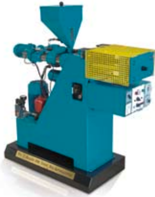
BOY 15 - the world's first injection moulding machine featuring the fully hydraulic two-platen clamping system, year of construction 1968
