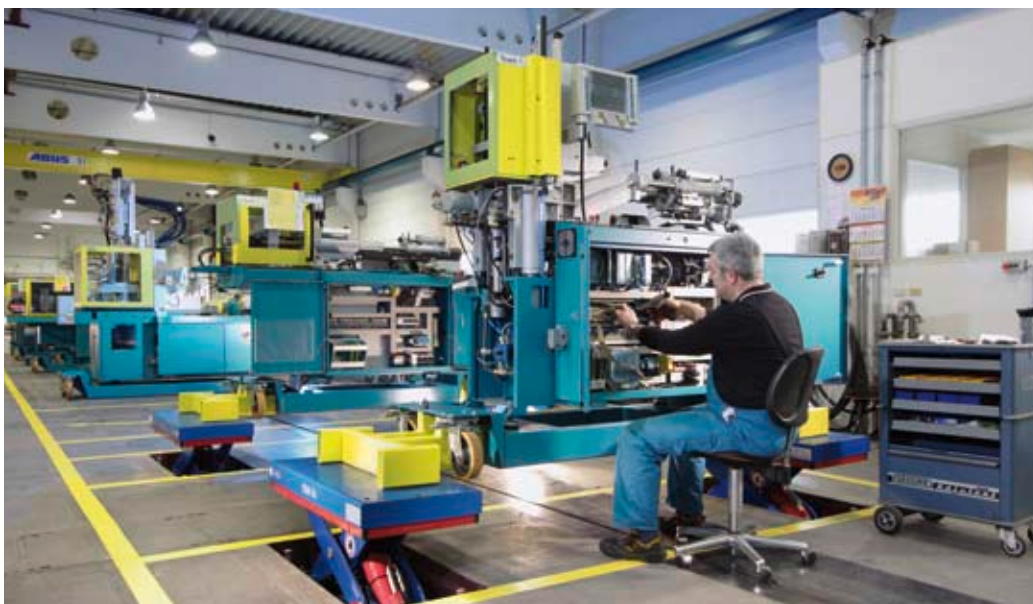
The state-of-the-art flexible flow production process allows machines to be transported on individual carriages to the necessary ergonomically designed assembly stations
